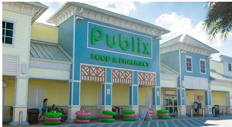
Figure 4.3.4: There should be no facade that has more than 100’ of run without a minimum 16” break in directional or material change.
